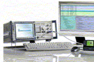
R&S®CMW500 wideband radio communication tester (base station simulator)
