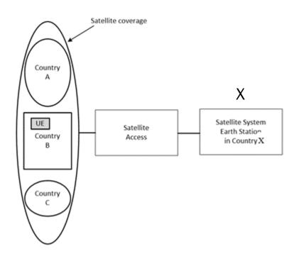
Figure 5.3-1 Satellite access with satellite beams overlapping several countries
