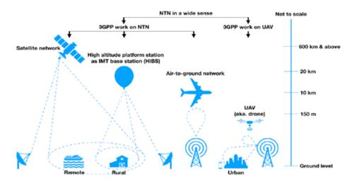
According to 3GPP TR 38.821<sup>17</sup>, the two typical scenarios of a satellite-based NTN providing access to user equipment are depicted below:
