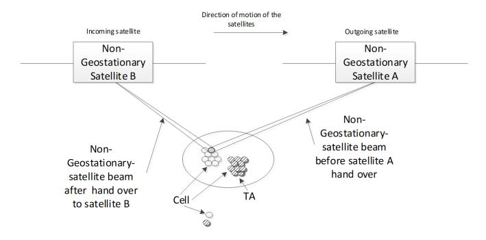
Figure 4.2-2 Non-Geostationary Satellite Beam steering and Handover (source: 3GPP SA2 study report 23.737)
