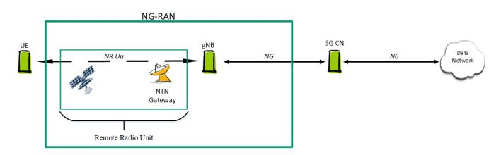
Hence the satellite repeats the NR-Uu radio interface from the feeder link (between the satellite-based NTN gateway and the satellite) to the service link (between the satellite and the UE) and vice versa. The Satellite Radio Interface (SRI) on the feeder link is the NR-Uu. In other words, the satellite does not terminate NR-Uu. The satellite-based NTN Gateway (GW) supports all necessary functions to forward the signal of NR-Uu interface.
