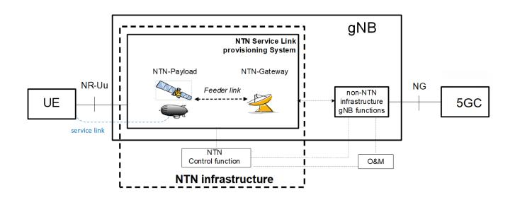
Treat "payload + feeder link + gateway + gNB" as essentially everything between Uu and Next Generation (NG) interface as a single entity, that may be called a "satellite access node" instead of "gNB". In this architecture, the interface between Satellite and Gateway, between gateway and gNB are not defined and may become proprietary.
