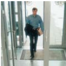
Compression level "low" Compression ratio 1:16 6% of original file size No visible image quality degradation
