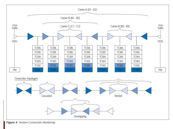
Each of the six TCMi fields in the ODU overhead is assigned to a monitored connection. There can be from zero to six levels or connections that can be configured for each ODU trail. In the Figure 4 example, there are three different levels that are actually monitored. Carrier C, due to its location, can monitor three TCM levels as the ODU passes through its portion of the network. The other carriers also monitor the levels according to agreement and location.
